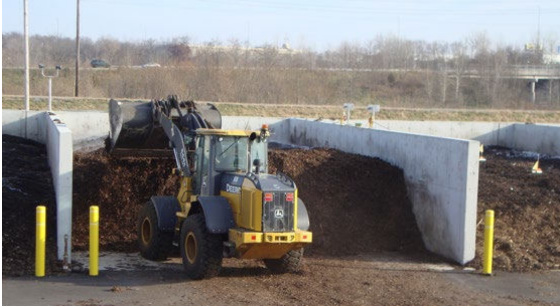
Photos 2 Heap composting using loaders to move the windrows
