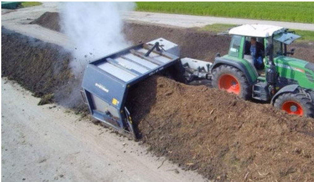
Photos 1 Heap composting using tractor pulled compost turners
